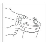
**Step 7**Place lid back to its proper position by aligning the arrow with the rear seam.
